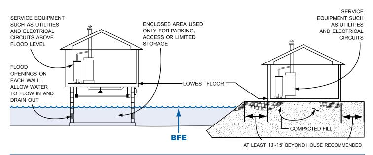
**Caution!** Enclosures (including crawlspaces) must meet special design requirements (see pages 43 and 44). **Note**: When the walking surface of the lowest floor is at the minimum elevation, under floor utilities are not allowed.
