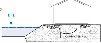
Fill slopes exposed to flood waters be protected from erosion by vegetation or stone armor depending upon anticipated water velocity.
