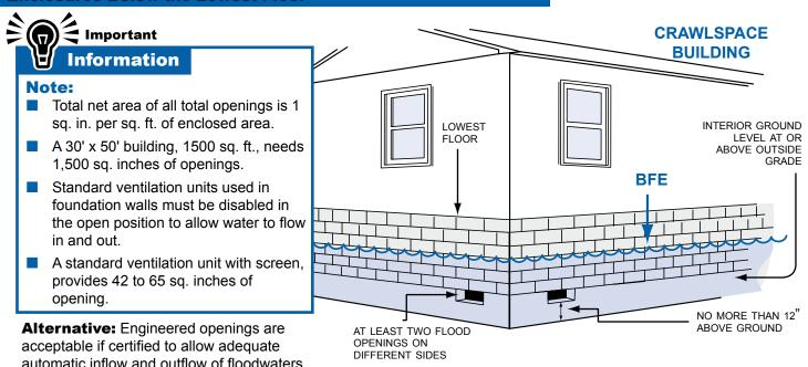
Solid perimeter walls can enclose floodprone areas. A crawlspace is a good way to elevate a few feet. In all cases the following are required: flood openings, utilities elevated to or above the BFE, two feet above BFE is recommended and is required in most communities, flood resistant materials and limitations on use of enclosures below the lowest floor. Check with the local permit office for details and restrictions.
