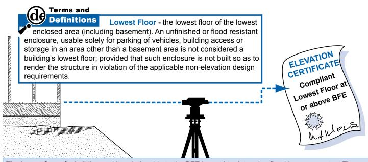
The lowest floor of a building and its relationship to the BFE is used to determine flood insurance rates. The lowest adjacent grade and its relationship to the BFE is used to determine if flood insurance is mandatory (previous page). If the lowest floor of a structure is at or above the BFE, a completed Elevation Certificate can be used to get lower cost flood insurance (see page 65). Two feet above BFE is recommended and is required in most communities.
