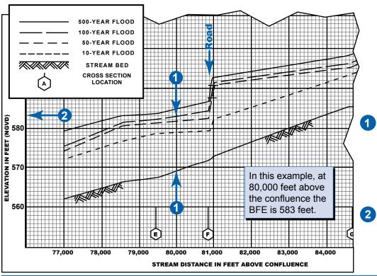
Flood profiles can be used to determine the BFE at a specific site. Profiles also show estimated water surface elevations for floods other than the 1%-percent annual chance flood.
