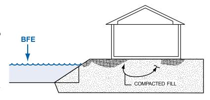
Your community may ask for certification of the elevation, compaction, slope and slope protection materials. Your engineer or design professional can find more information in FEMA's technical guidance for Letters of Map Revision based on Fill (FEMA Form MT-1) and in NFIP Technical Bulletin #10.
