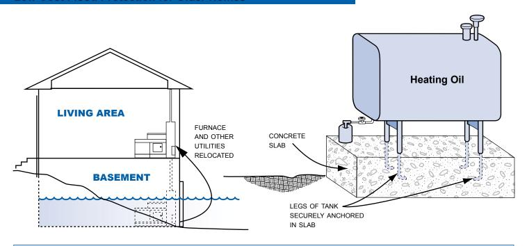
Move your water heater and furnace out of the basement, or build small elevated platforms for them. If the flood depth is less than two feet, build flood walls or anchor the tanks. **Do not** store valuables in a floodprone basement. Use flood resistant materials when you repair.
