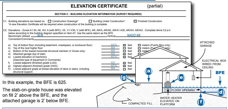
You must have a surveyor licensed to practice in Tennessee, complete the Elevation Certificate and seal it. The Elevation Certificate includes diagrams for ten building types. Several points must be surveyed.
