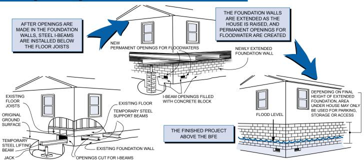
This is one way to elevate an existing building to comply with floodplain regulations. See *Above the Flood: Elevating Your Floodprone House* (FEMA 347) for additional information. If your insured building is damaged by flood and your community determines it is substantially damaged, you may be eligible for an **Increased Cost of Compliance** payment (see page 63).
